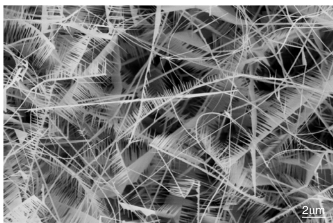
Figure 10. An SEM image of ‘comb-like’ cantilever arrays of ZnO, which are the result of surface polarization induced growth due to the chemically active (0001) Zn (image courtesy of Dr X Y Kong) [22].
